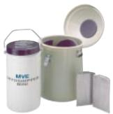
The unique cryo-block inserts enable the user to optimize hold time and capacity. Available in three sizes 1, 1.5, and 2 inches, each pair of blocks provides a specific hold time between 2 and 8 days.
